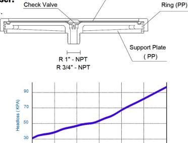
Specific air load of the OXYaero - D270 membrane disk diffuser
